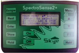
Logging display meter for visible/NIR light sensors Incident & reflected light measurements Matched to satellite wavebands Direct readout of NDVI Logging of measurement location via GPS
